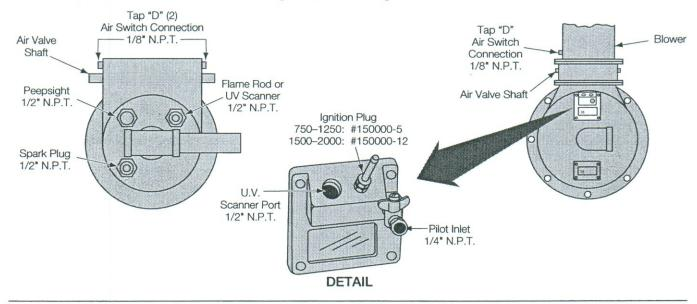
Figure 5-Blower Motor Replacement
