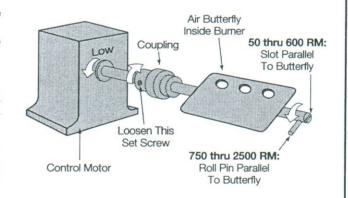
Note: Arrows apply to motors which rotate counterclockwise to low fire. Reverse all arrows for clockwise motors.
